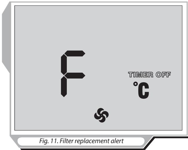
Fig. 11. Filter replacement alert
