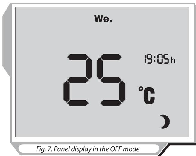
Fig. 7. Panel display in the OFF mode
