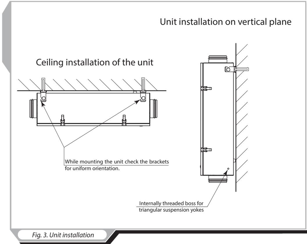
The absence of a drain pan in the unit enables its installation in any position provided unhindered access for maintenance. For best unit performance connect a straight duct section at least 1 m long on both sides of the unit.
