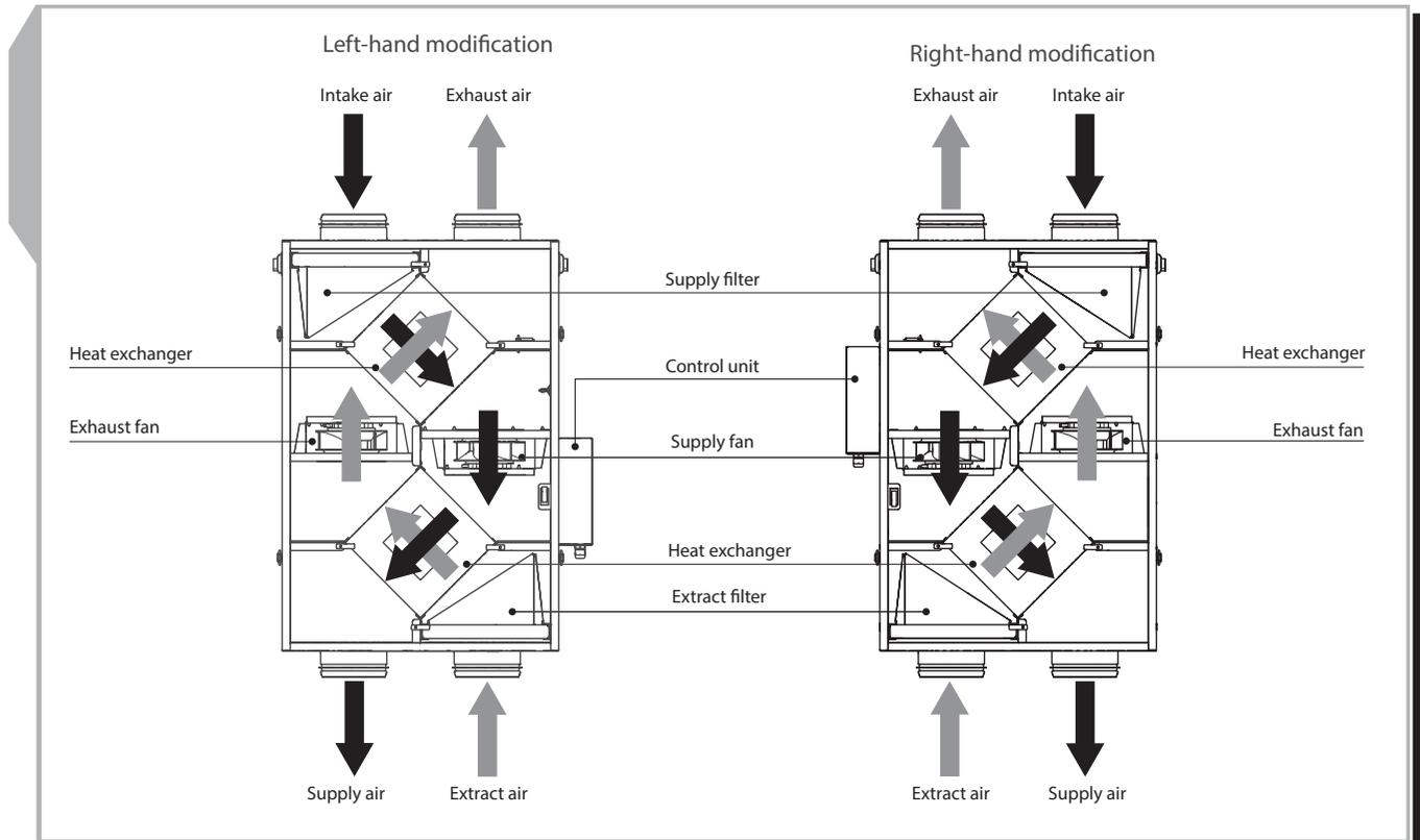
Fig. 2. Design and operating logic
