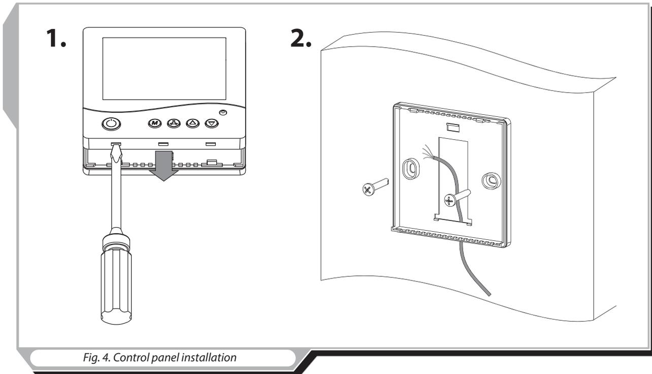
Fig. 4. Control panel installation
