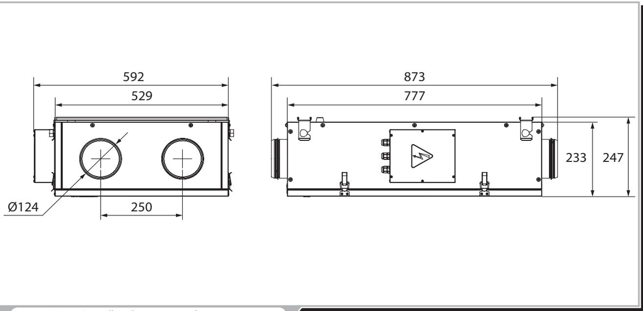
Fig. 1. Overall and connecting dimensions
