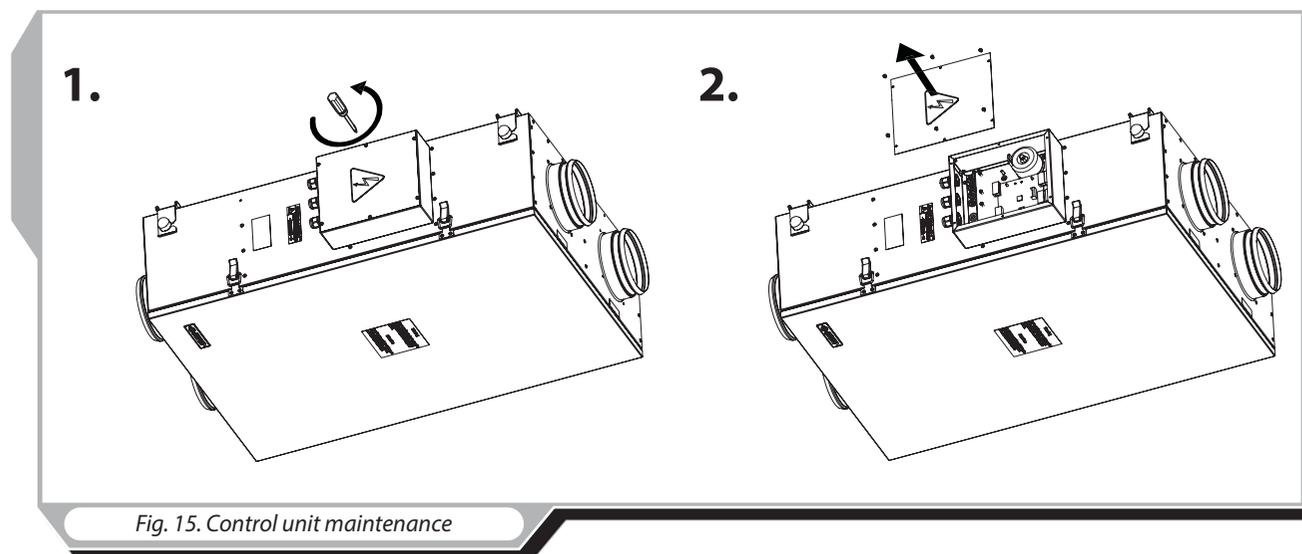
Fig. 15. Control unit maintenance
