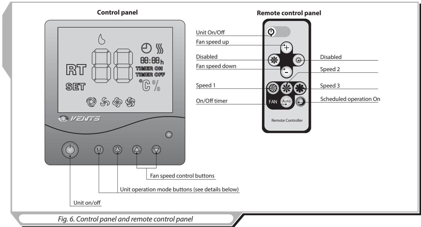
The unit is controlled by means of the remote-mounted control panel and the remote controller (Fig. 6).
